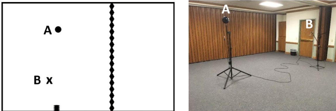
FIG. 2.11. (left) Source A and receiver B locations in a medium room configuration with one room divider closed and the other open. (right) a photograph representing this same configuration where A is the location of the dodecahedron sound source and B is the location of the random-incidence microphone.
